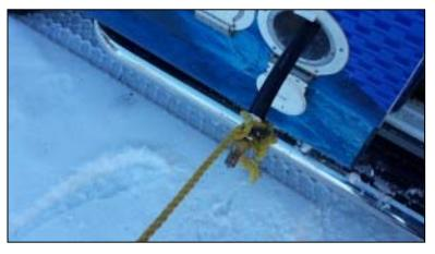
11) Quick connector wraps if you are using shorter high pressure hoses. I really recommend for winter especially getting a longer amount of **uninterrupted** high pressure hose. Hoses tend to freeze at the connectors.
